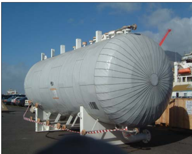
Process vessel clad with ULVA Shield prior to shipment from Canada to The Caspian Sea.
